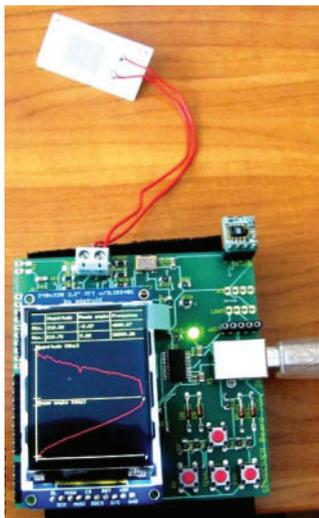
Fig. 3 A hardware outcome of Control board with connected sample under test
