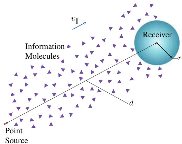
Fig. 1: Molecular communication system via diffusion with flow (or drift).
