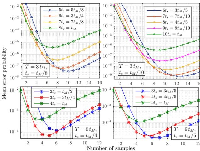
Fig. 8:  $P_e$  for various values of  $T$ ,  $t_s$  and  $t_1$ , where  $v = 1$  mm/sec and  $\mu_N = 500$ .
