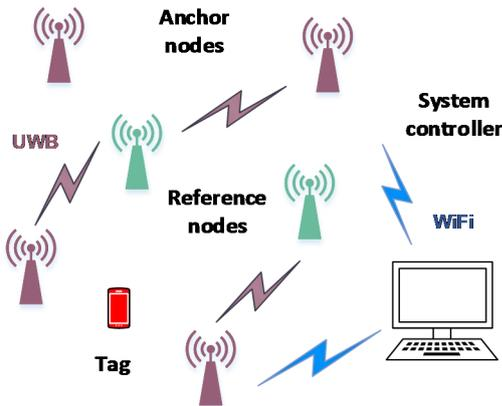
Fig. 1. Proposed architecture of the UWB localization system
