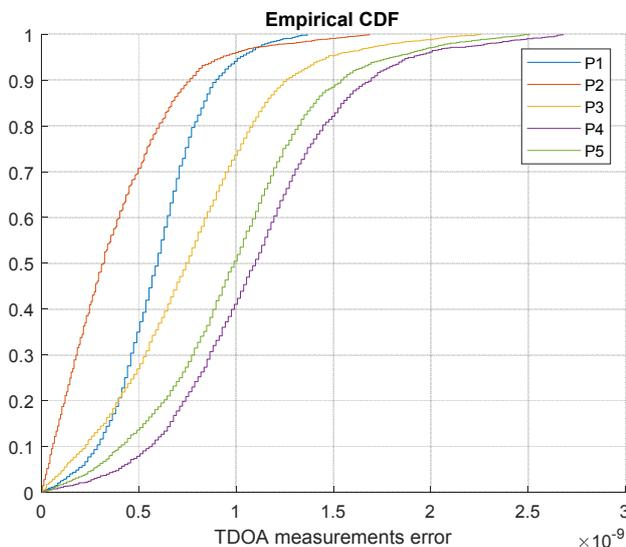
Fig. 5. CDF of errors of TDOA measurements (AN1 synchronized to R1, AN2 to R2)
