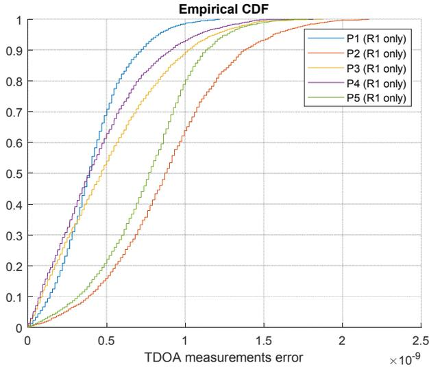
Fig. 4. CDF of errors of TDOA measurements (both anchors synchronized with R1)
