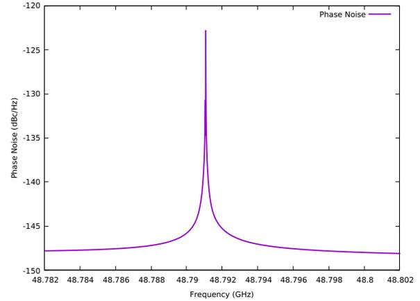
Fig. 6. 48.8GHz Oscillator Phase Noise
