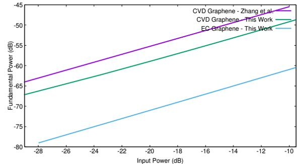
Fig. 7. x2 GFET Subharmonic Mixer Fundamental Power [24]
