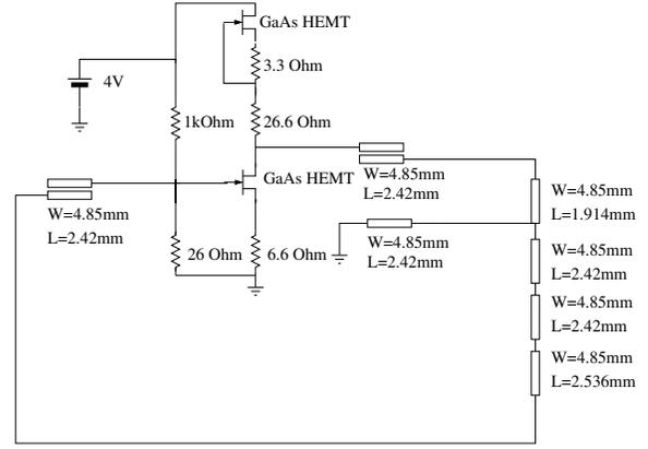
Fig. 1. Low Phase Noise 24.4GHz GaAs HEMT Oscillator
