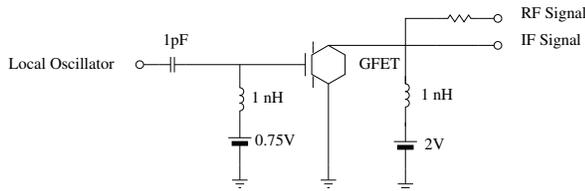
Fig. 3. 10 $\mu$ m Electrochemical GFET x2 Subharmonic Mixer
