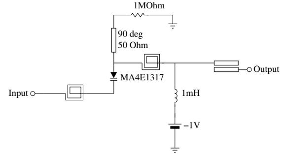
Fig. 2. Schottky Varactor Frequency Doubler - 24.4GHz to 48.8GHz
